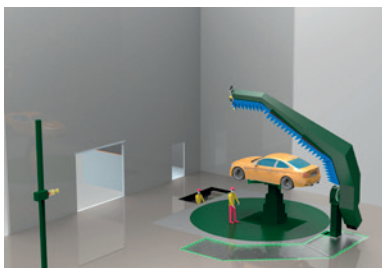
Gantry arm integrated in a combined NF/FF automotive test range
